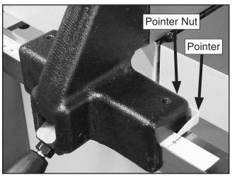
**Figure 12**. Calibrating fence pointer (screw out of view).
